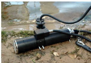
Benthofluor analysis of benthic algae, can be used as a FluoroProbe
